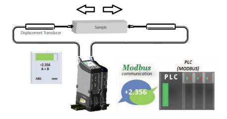
Use 2 S-Series Transducers to monitor a sample under strain
