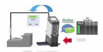
Simple height check measurement to PLC via MODBUS
