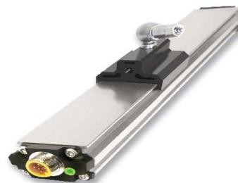
The S955 Brik linear displacement transducer is an economical solution for monitoring continuous position. It is designed for OEM users wishing to opt for a cost effective alternative to limit switches, proximity sensors or linear potentiometers. The streamlined anodized aluminium extrusion houses the sensing element and the electronics. The position is determined by the magnet which is linearly guided over the sensing element.
