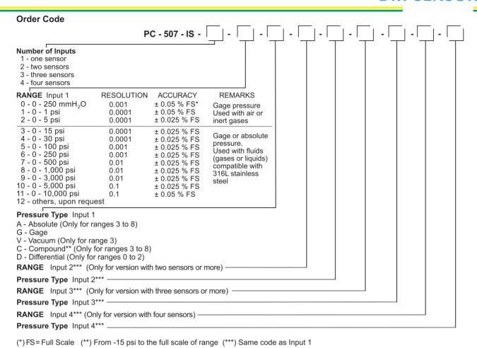
Code example: PC-507-IS-4-2-G-3-V-5-G-8-A, defines a four sensors calibrator, which input 1 range from 0 to 5 psi (gage pressure), input 2 from 0 to 15 psi (vacuum), input 3 from 0 to 100 psi (gage pressure) and input 4 from 0 to 1,000 psi (absolute pressure).
