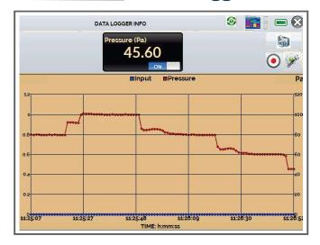
PCON-Y18-LP allows you to record series of measurements overtime to display in chart or table format.
