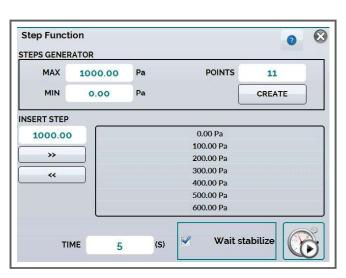
Predefined steps can be easily defined (division of span by a defined number of points, or values defined by the user). These steps are automatically executed by the pressure controller respecting the defined step duration.
